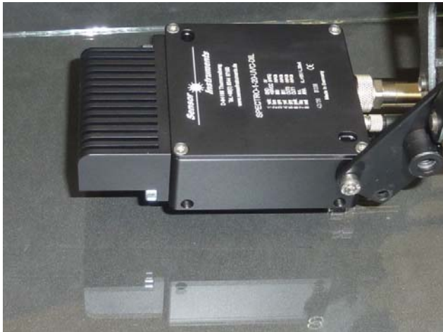
SPECTRO-1-20-UVC-DIL sensor, aimed at the tin side of float glass
