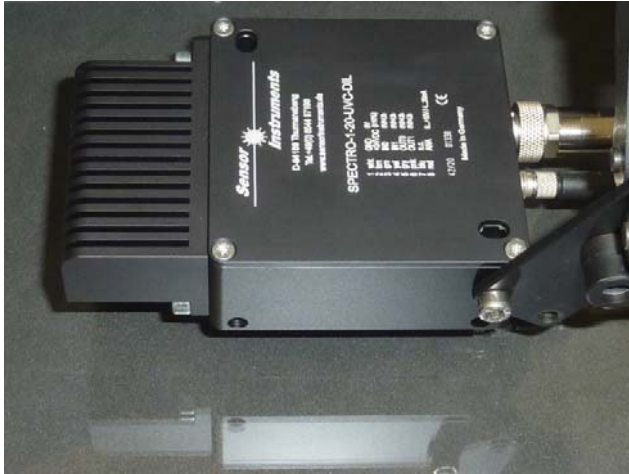
SPECTRO-1-20-UVC-DIL sensor, aimed at the fire side of float glasses from a distance of 20mm
